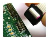
Connect the CC Debugger to the target. The minimum connection required for SoC debugging and programming is shown in the figure to the right.
