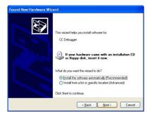
The PC will detect a new USB device when the debugger is connected to the PC. Windows will associate the device with a USB driver installed on the PC. When prompted, the driver installation/association should be handled automatically. If requested, the driver is located in C:\Program Files\Texas Instruments\Extras\Drivers
