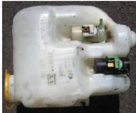
Figure 3—Option for Reservoir (2-pump)
