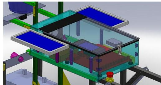
Figure 11 - 3D CAD Model of Electronics Box
