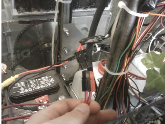
Connecting this will provide the board with power, and the regulators will step the 12V down to 5V and 3.3V for the electronics.
