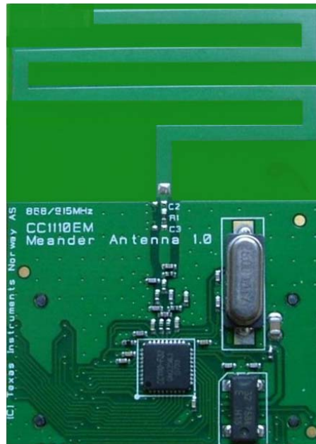
Figure 1. Prototype Board for 868 MHz, 915 MHz, and 955 MHz PCB Monopole Antenna
