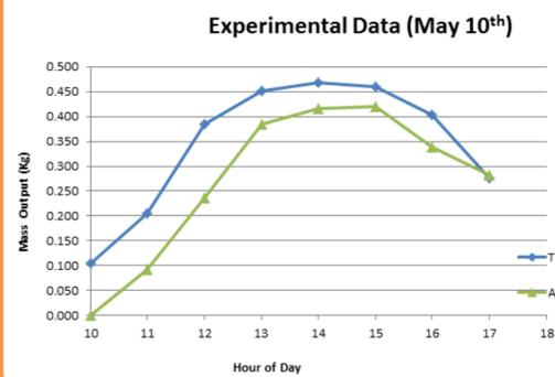
The main cause for the difference between the theoretical and the experimental is that the input solar insolation was less for the theoretical data, causing a lower system temperature.
