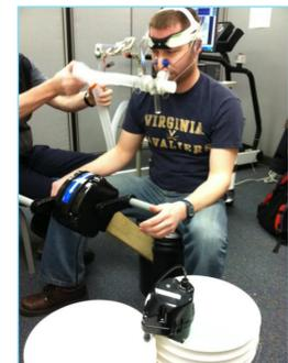
Figure 4: V<sub>O2</sub> Test Set-up
