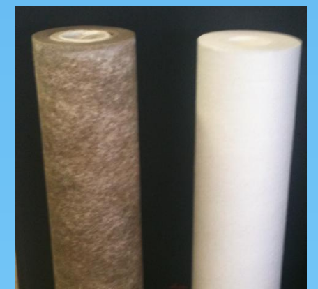
Paper filter before and after 8 minutes of run time
