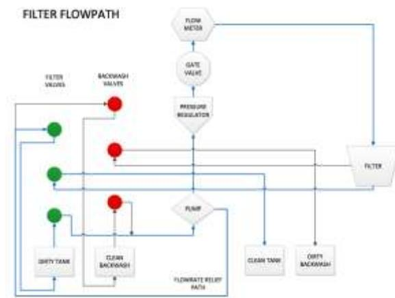
Figure #: Filter Flow Path
