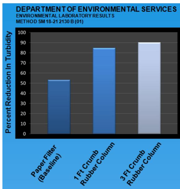
Figure 9: Turbidity Testing Results
