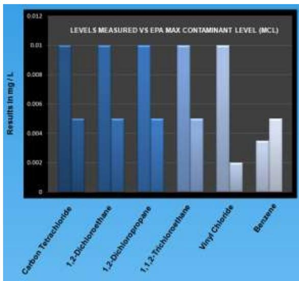
Figure 7: Volatile Organic Compounds in filtered water
