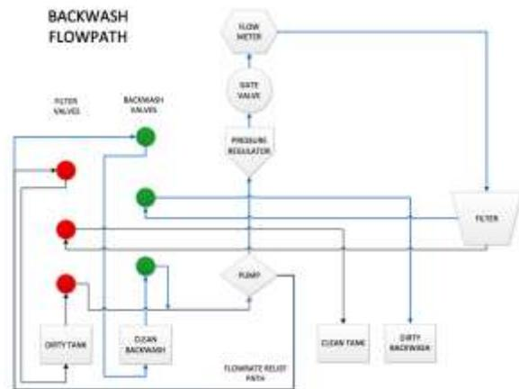
Figure 4: Backwash Flow Path
