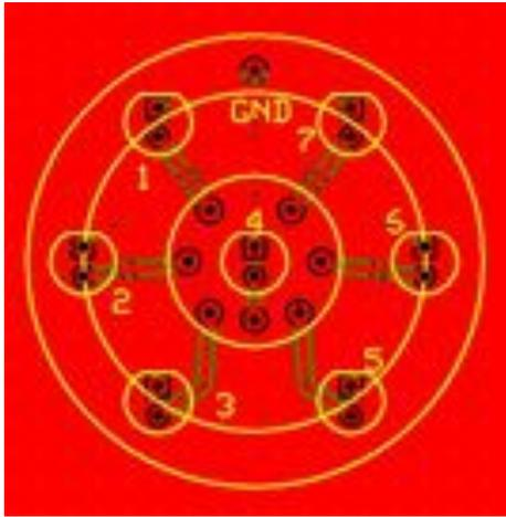
Figure 5. Original Cluster PCB Design (with Silk Screen)
