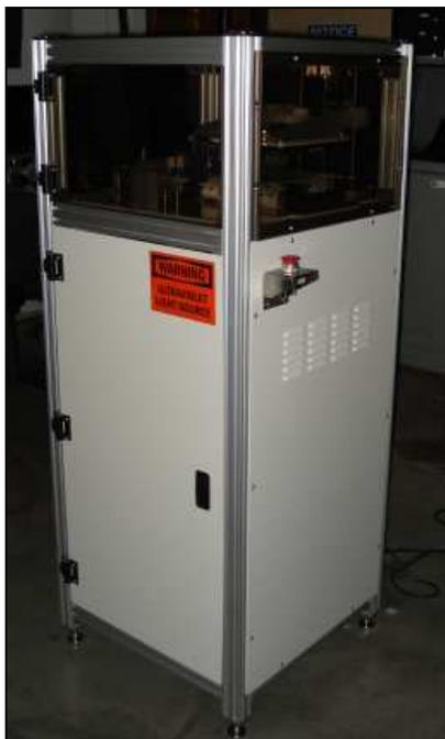
**Figure 9: DLP Prototyping System Frame**
