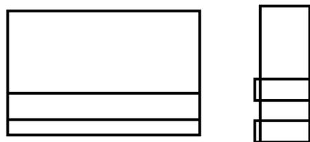
Figure 1.2 Voice Coil core (right final wrapped core with paper barriers, left starting piece of paper to be wrapped around a pole then add strips of paper for barriers)
