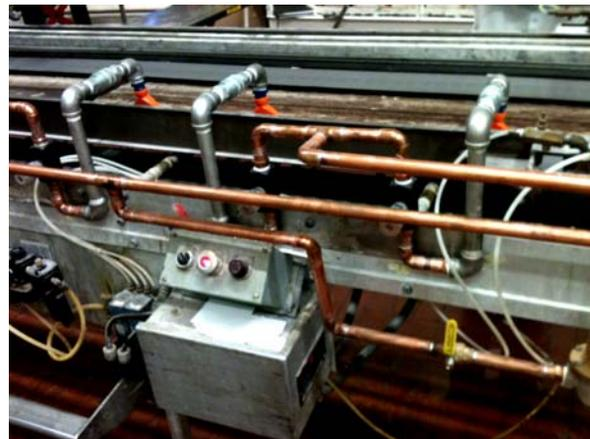
Figure (7) General overview of the system with piping and dispense heads.
