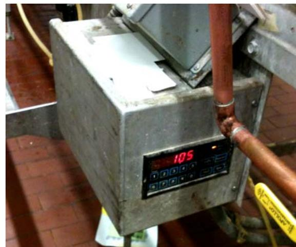
**Figure (11) Pulse counter in place for the conveyor belt set to 105 pulses for the pan catcher to trigger.**
