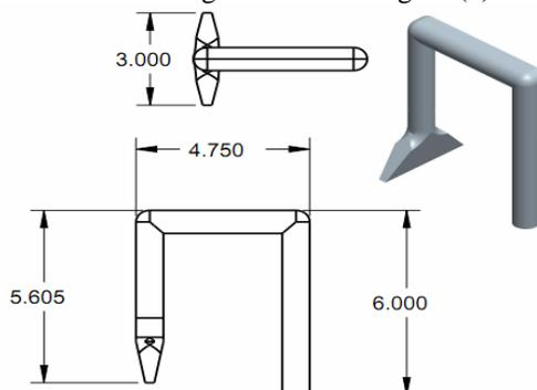
Figure (3) Elevated Water Outlet (Inches)
