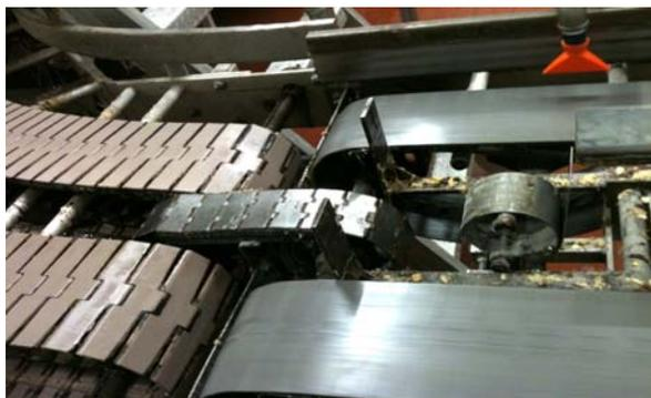
**Figure (9) Pan Stopper rises from the conveyor belt to stop pans from moving further.**
