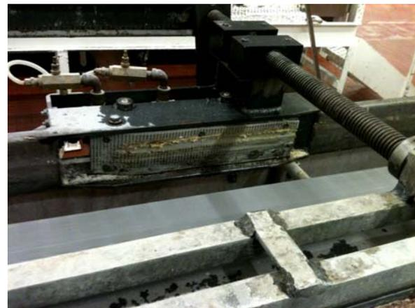
**Figure (10) Pan Catcher stops the 9th pan after the pulse counts to 105.**
