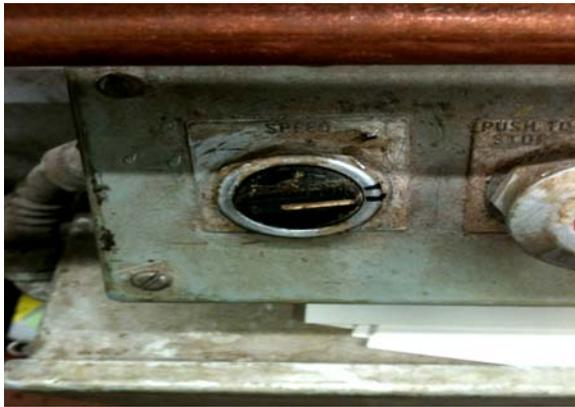
**Figure (8) Speed adjustment control with lower marking at 30 Hz and higher at 35Hz**
