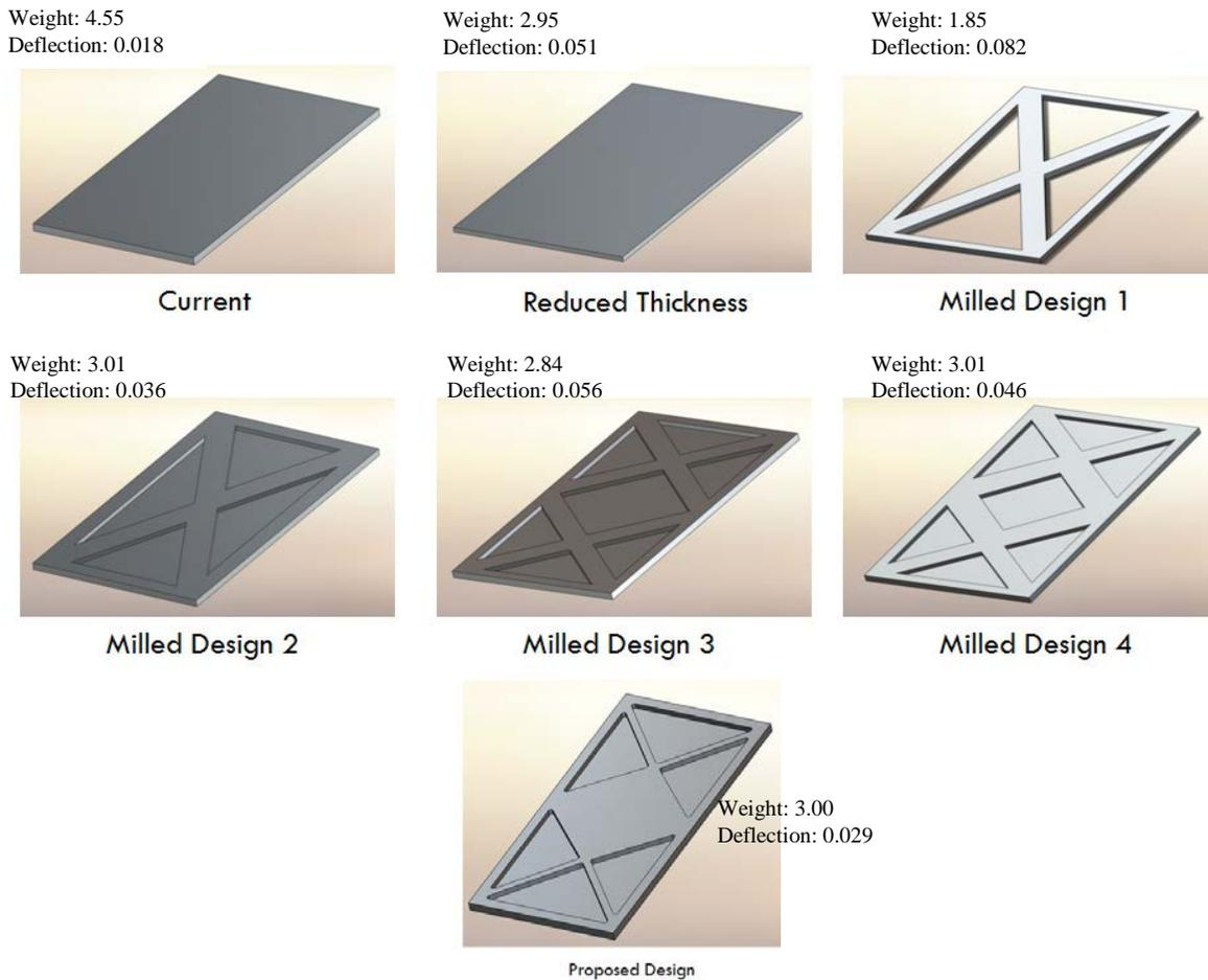
**Figure 5: Possible Designs for Foot Plates**
