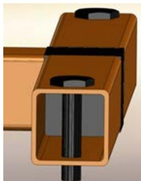
**Figure 9: Feet Design for Camera Structure**
