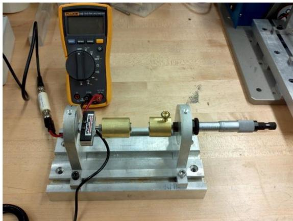
**Figure 3: Magnet Pull Force Setup**
