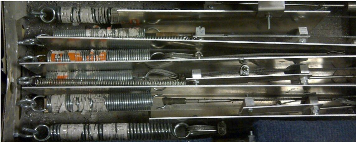
*Figure 5: Spring Feedback System*
