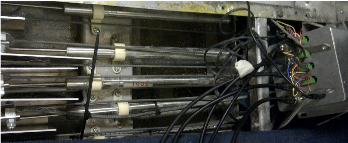
*Figure 4: LVDT Connection System*
