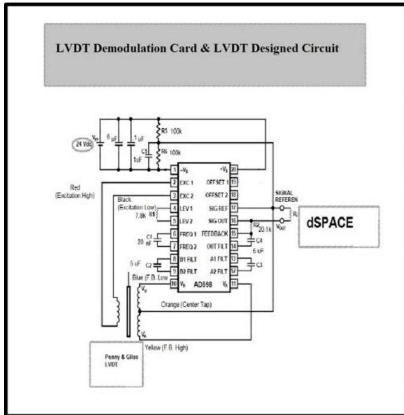
Figure (8) – LVDT Demodulation Circuit
