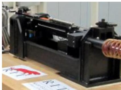
*Figure (4) – Donated Test Rig Base Platform*
