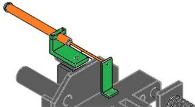
Figure (7) – LVDT Mounting System
