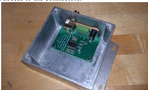
*Figure (10) – Demodulation Card in Enclosure*
