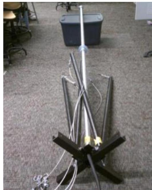
6. Connect the two (2) turbine assembly electrical connectors (assembly 3) to the two (2) electrical connectors on the cable protruding from the top of the mast as shown. The connectors are male-female and female-male and will only connect one way. **DO NOT FORCE THE ELECTRICAL CONNECTORS TOGETHER.**
