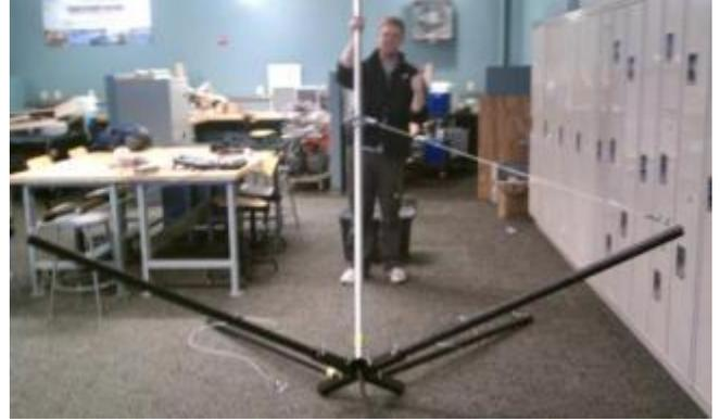
16. While raising the stand, the lower two legs will fold out into place. Once the stand is fully erect, with one person holding the mast in place, the second person can attach the remaining two guy wire hooks to their respective holes in the guy wire flange, and reinstall the outer leg pins through the remaining two legs.
