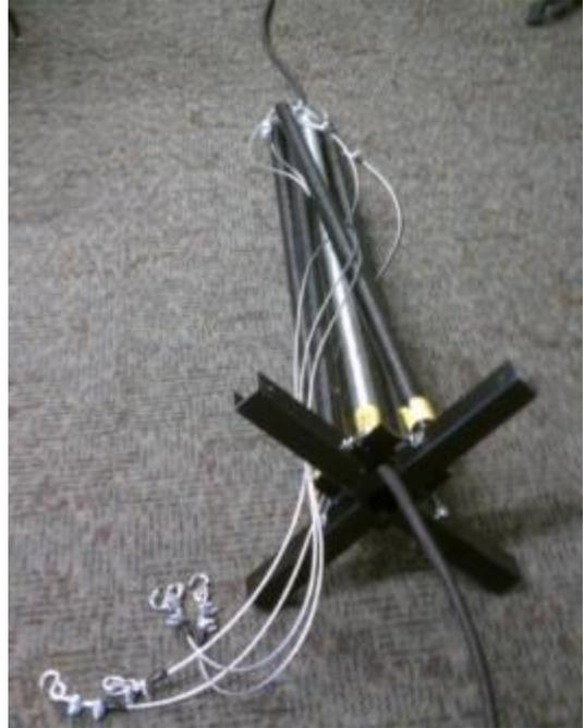
3. Insert the end of the electrical cable with two connectors through the coupling end of the upper mast, assembly 2, and pull through
