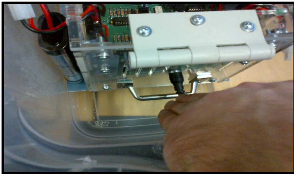
Figure 4 - Connecting the P12401 Power Barrel Connector into the P12402 Port
