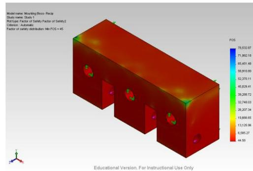
**Figure 5: Compressor Mounts FEA**
