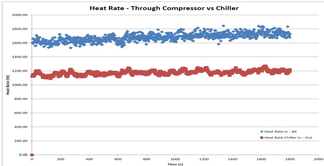
Figure 8: Initial Heat Rate Data Through Compressor
