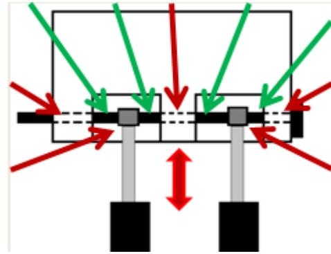
**Figure 12: Original MR Damping System: Green Arrows Indicate Bending, Red Arrows Indicate Tolerance Stackup Locations**
