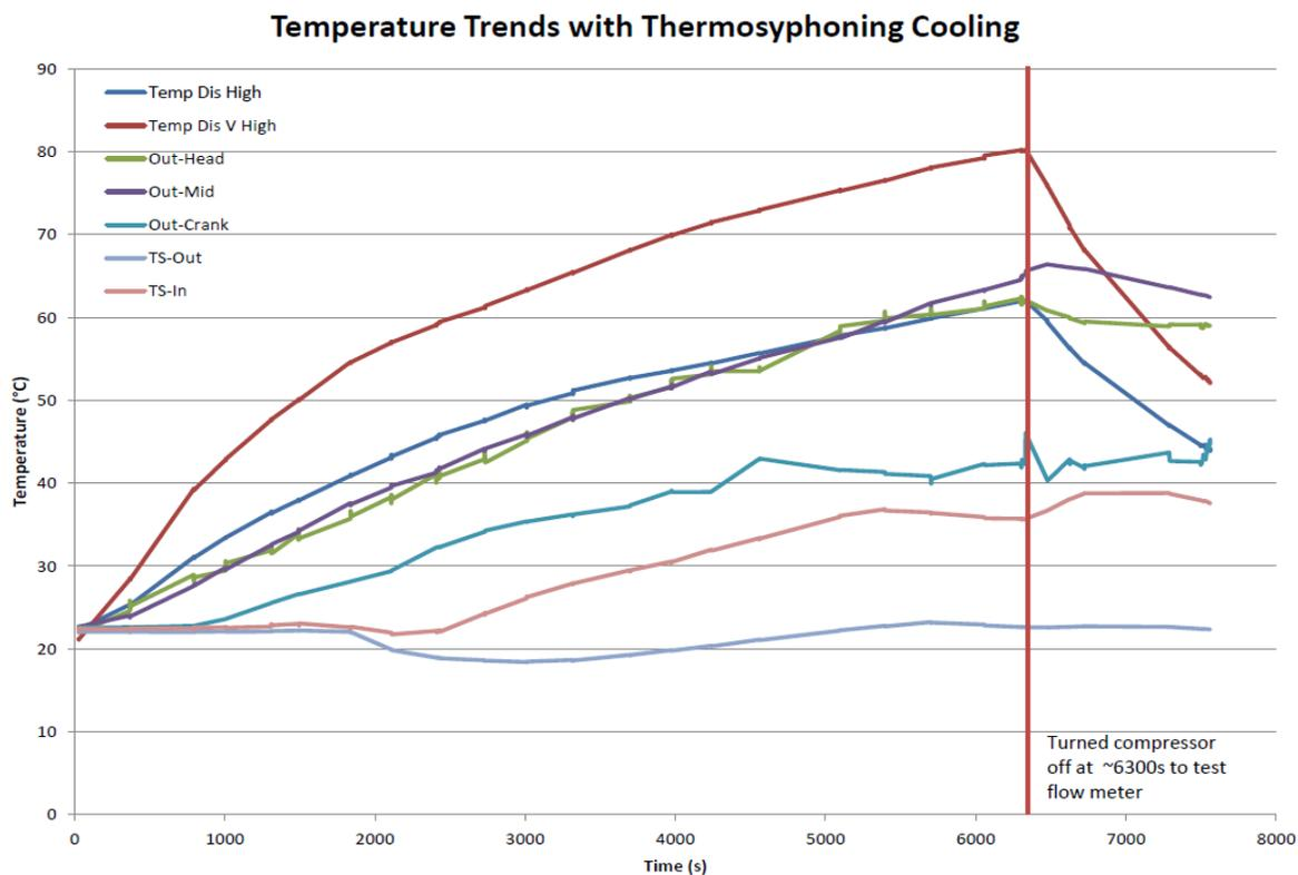
**Figure 11: Temperature Trend Data for Compressor with Thermosyphoning Cooling System**
