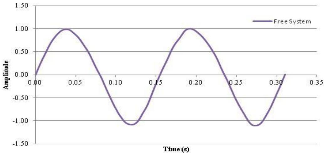
Figure 7. Normalized acceleration amplitude versus time for the initial, undamped system.
