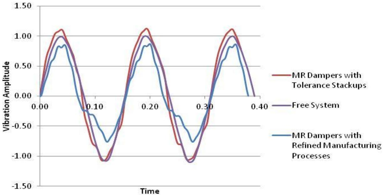
Figure 10: Normalized Acceleration Comparison of Undamped System, MR Dampers with tolerance stackups, and revised MR Damping System
