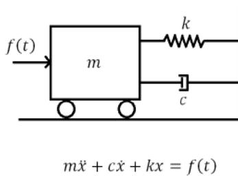
**Figure 4: Spring-Mass-Damper Model of Compressor System**
