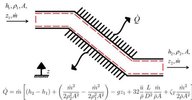
**Figure 6: Control Volume for Thermosyphoning Analysis**
