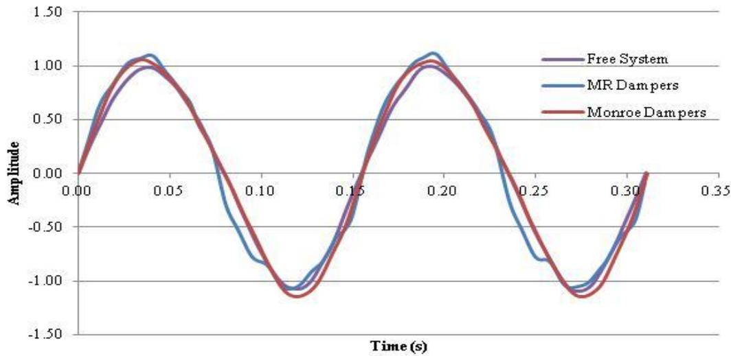
Figure 9: Normalized Acceleration Comparison of the Undamped System, MR Dampers, and Automotive Dampers
