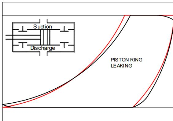
Figure 1: Difference between healthy (red) and faulty (black) P-V diagram [1]
