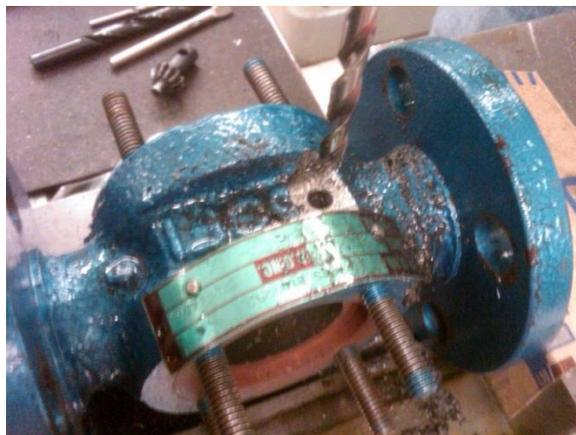
Figure 2: Example of modifications to existing structure necessary to accommodate sensor installation
