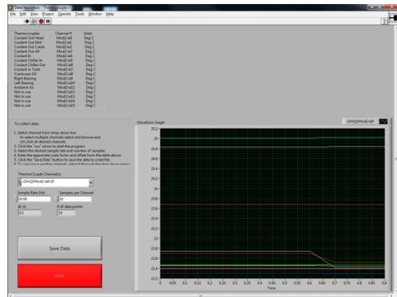
Figure 5: Thermocouple channel data collection
