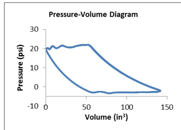
Figure 8: P-V Diagram of the compressor
