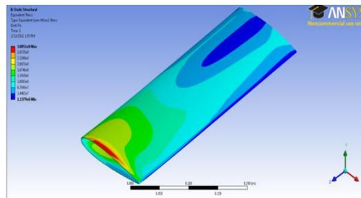
Figure 4: Hydrofoil fiberglass layer in ANSYS
