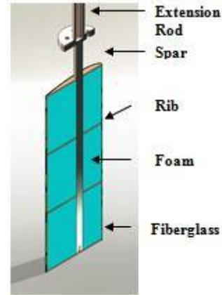
Figure 1: Hydrofoil section view
