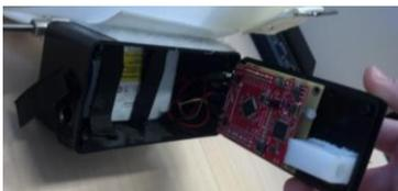
Figure 3: Main printed circuit board on top portion of electronics enclosure with the battery in base of enclosure.
