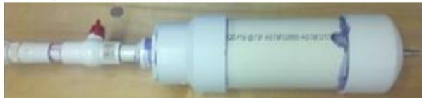
Figure 6: First iteration of tank design constructed as a proof of concept for high air flow concept.
