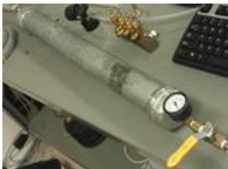
Figure 7: Second iteration of tank design created a safer testing environment with accurate pressure readouts.
