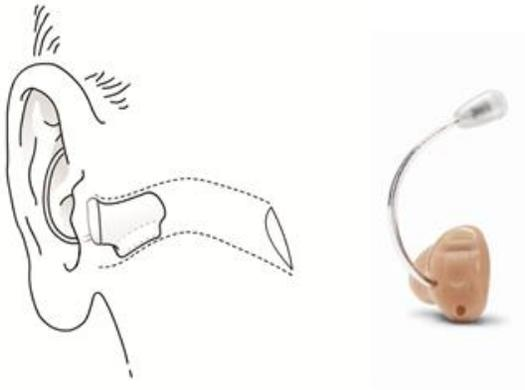
**Figure 1.** In the RM design, the placement of the microphone in the concha cymba hides the microphone not only for improved cosmetics but also for improved acoustic performance due to pinna effects and protection from turbulent wind noise.
