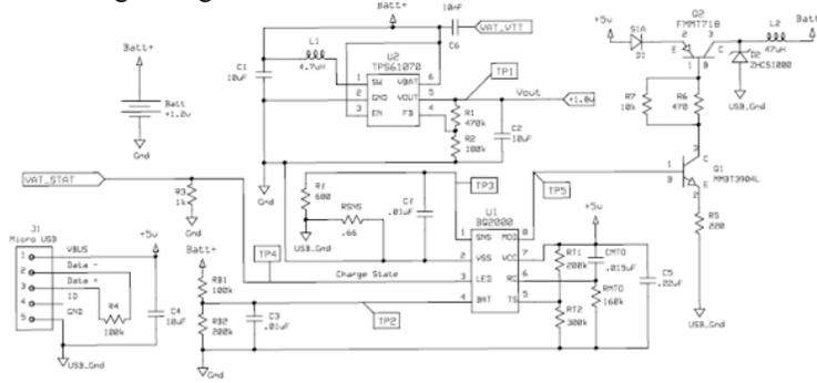
Figure 6: Battery Charging Circuit Schematic
