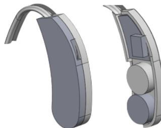
**Figure 5: Battery Enclosure**
