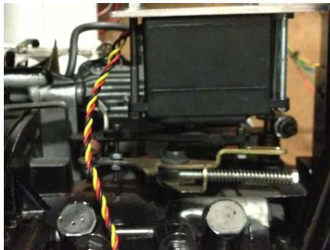
Figure 3 Throttle Servo attached to the Motor Control Arm
