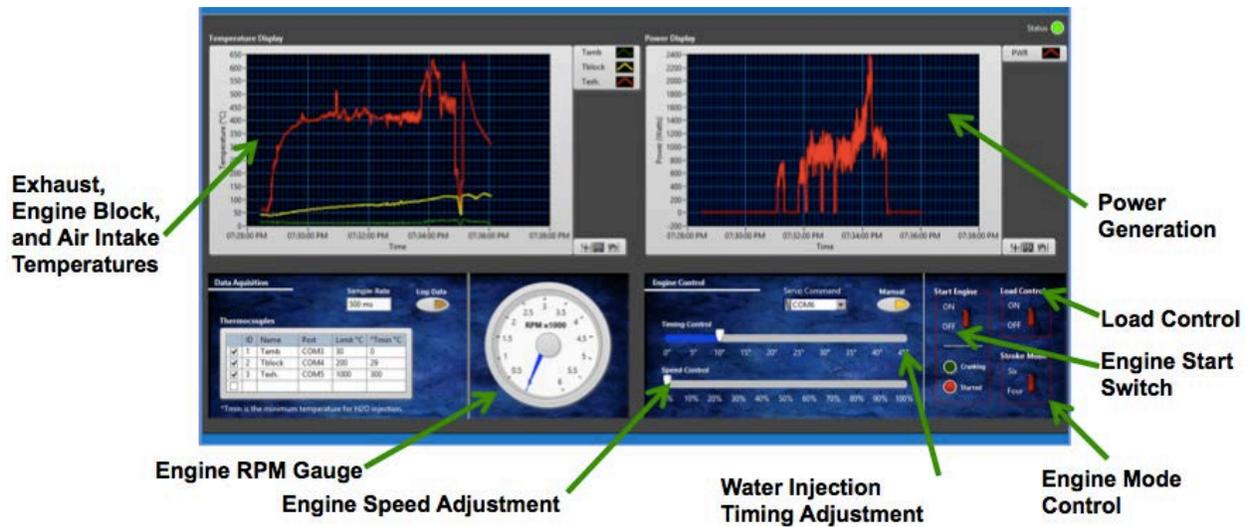
Figure 2 LabVIEW Graphical User Interface (GUI)
