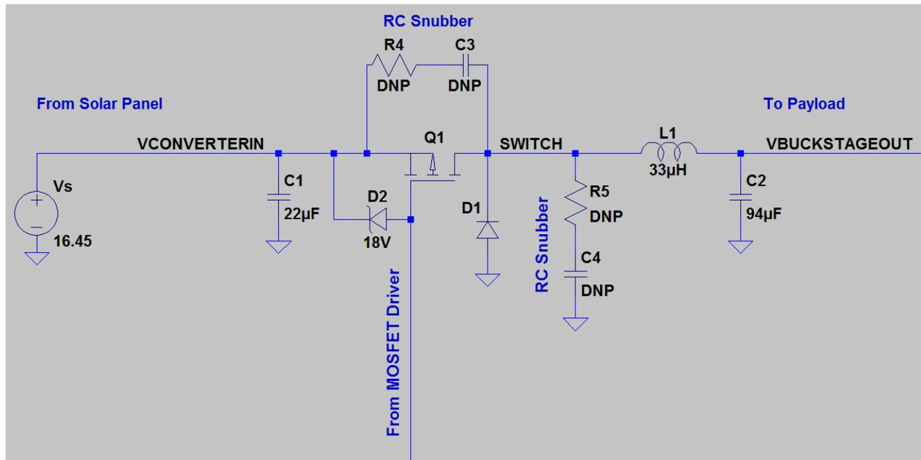
Figure 1: The step-down "buck" converter schematic with test circuitry used in simulations.
