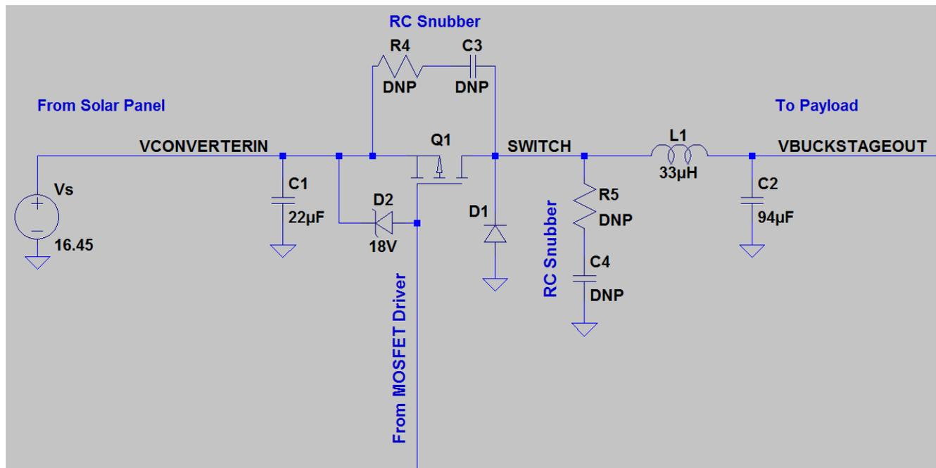
Figure 2: The DC/DC buck converter that provides energy to the output of the MPPT. Used for reference only.
