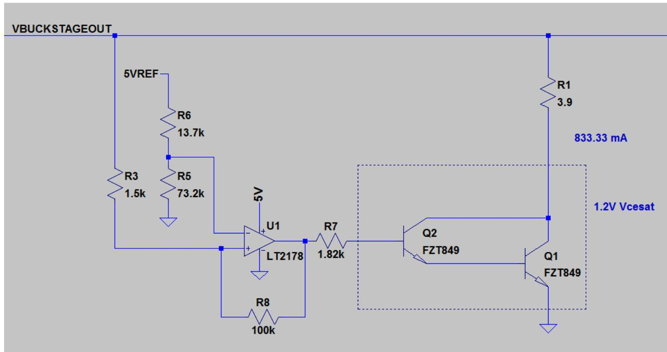
Figure 1: The output voltage clamp schematic that is intended to protect the payload from voltages above the 4.1V limit. Comparator U1 implemented with an op-amp to slow the response down. Devices shown in this schematic are for reference only.
