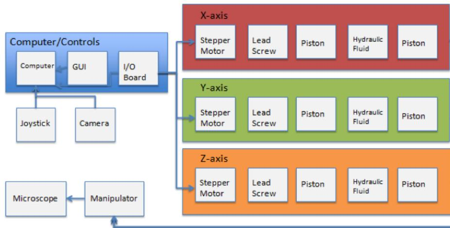
Figure 02: System Architecture
