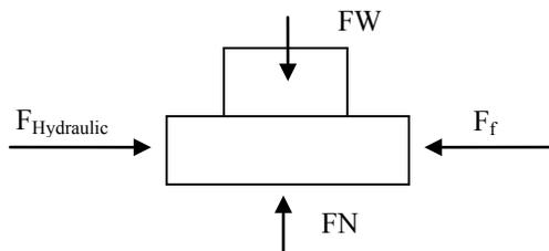
Figure 05: Stack Up of Three Axis and Forces Experienced by Carriage
