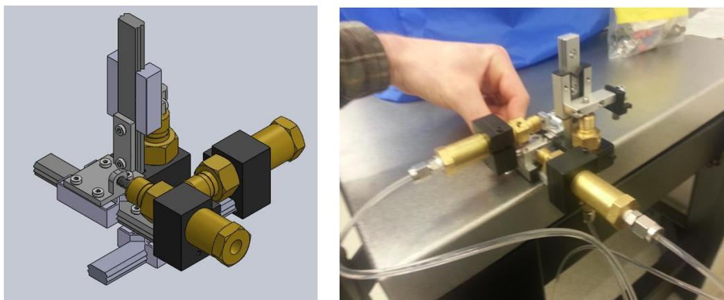
Figure 06: Manipulator Assembly in CAD and Hardware
