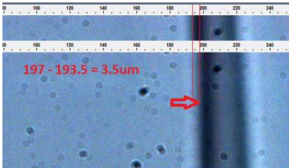
Figure 6: The above figure shows the pipette position before (above) and after (below) resolution testing. Motion can be observed with reference to the point change in position of the red line.
