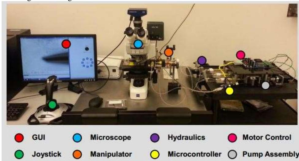
Figure 2: The nanomanipulator system and its subsystems. [2]
