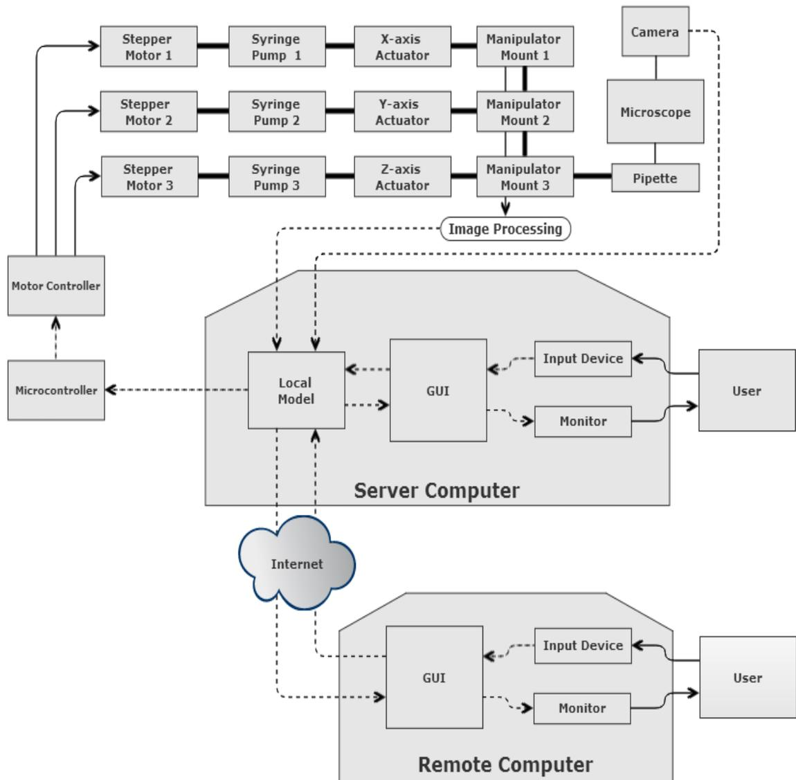
Figure 4: The proposed nanomanipulator system architecture.
