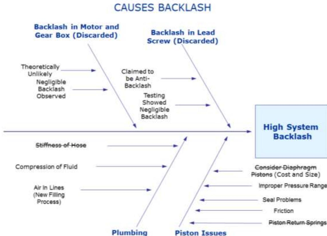
Figure 5: A fishbone diagram highlighting possible areas of improvement on the original system.
