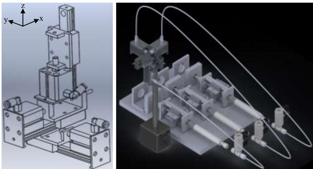
Figure 1: CAD model of manipulator system, with a system assembly drawing using the old mounting configuration
