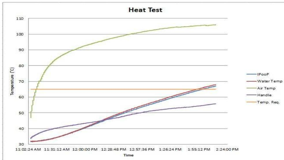
**Figure 8: Plotted Temperatures from the Heat Test**
