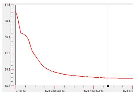
**Figure 6: Pillar Wax with Melting Temperature of 58.8 °C**
