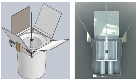
**Figure 7: Waste Pasteurizer Isometric View (left) and Cross Sectional View (right)**
