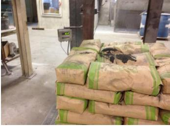
Using pallets to distribute the load 50lb bags were added until an anticipated break. When the weight exceeded 1600lbs it was deemed safe and strong enough for the constraints. Also, with the weight on it an individual climbed on the stacked bags and shifted their weight back and forth. Although the frame gave a little it showed no signs of permanent stress or break.
