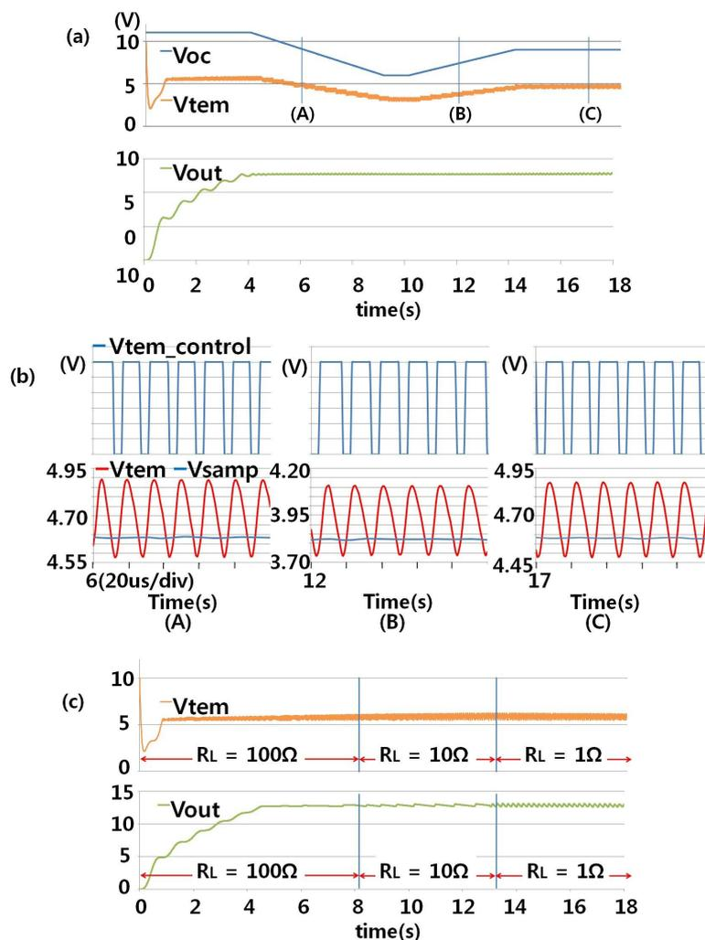
**Fig. 2.** (a) SPICE simulated voltage waveforms of the proposed MPPT circuit with load resistance of 5 W. (b) Voltage of comparator output ( $V_{tem\_control}$ ),  $V_{samp}$ , and  $V_{tem}$  at the timing of (A), (B), and (C). (c) Simulated voltage waveform of  $V_{out}$ ,  $V_{tem}$  and  $V_{samp}$  against abrupt change of  $R_L$  while  $V_{OC}$  is fixed at 11 V.
