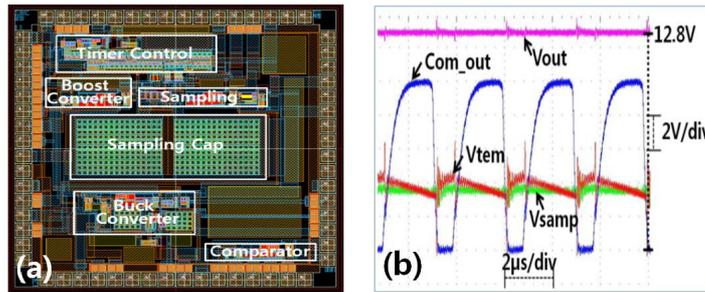
**Fig. 3.** (a) Layout view of the fabricated Chip with area of  $3\text{ mm} \times 3\text{ mm}$  (b) Measured voltage waveforms of the  $V_{\text{out}}$ , comparator output,  $V_{\text{samp}}$ , and  $V_{\text{tem}}$
