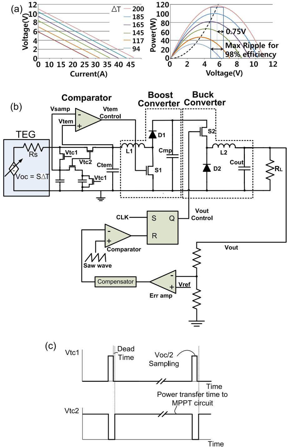
**Fig. 1.** (a) Measured voltage versus-current characteristics and Power versus voltage characteristics of a Bi<sub>2</sub>Te<sub>3</sub> thermoelectric module. (b) Proposed MPPT circuit employing the boost cascaded-with-buck converter with feedback circuit for constant output voltage. (c) Waveforms of  $V_{tc1}$  and  $V_{tc2}$  sample and hold timing signal
