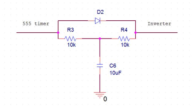
Figure 3: The delay network to create dead time.
