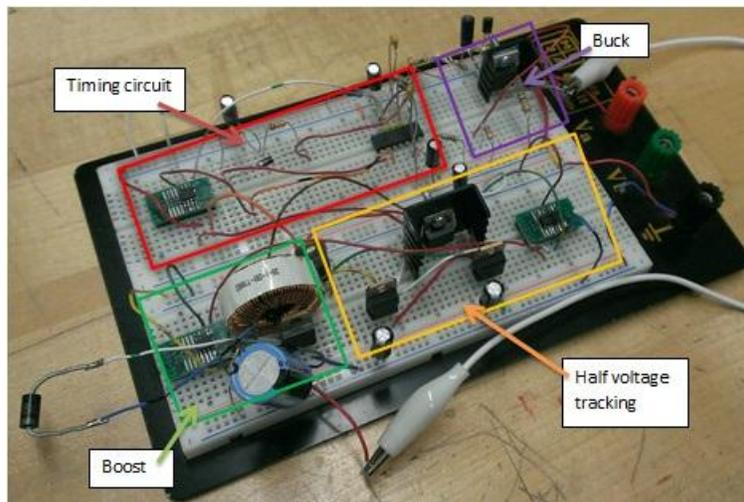
Figure 2: MPPT prototype
