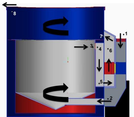
**Figure 3: Conceptual stove cross-section with air flow path and points of interest**
