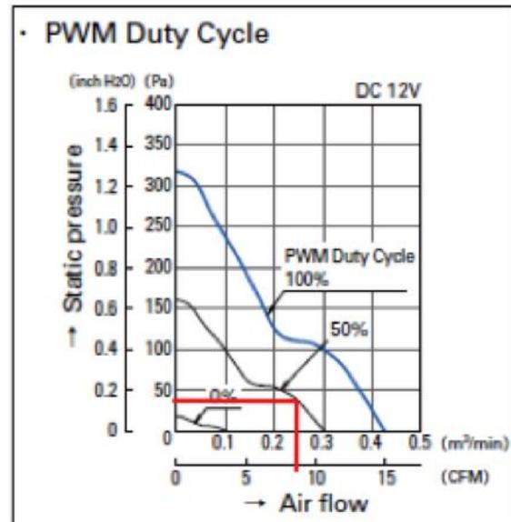
Figure 4: Fan operating curve
