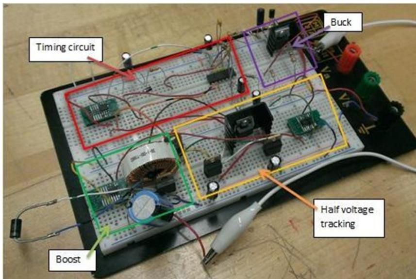
**Figure 6: Physical Layout of MPPT**
