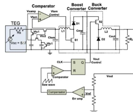
Figure 5: Layout of the MPPT circuit
