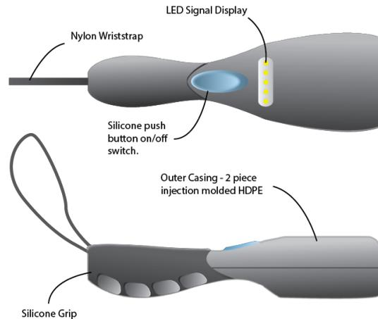
Figure 1 - Conceptual design of leak detector detailing interactive features
