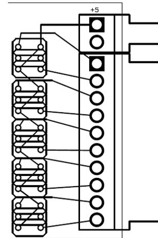
Figure 5 - Final LED Display layout
