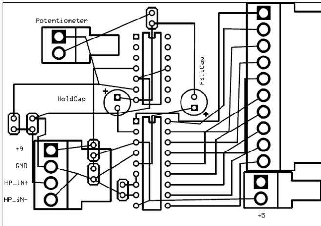
Figure 4 - Final PCB layout
