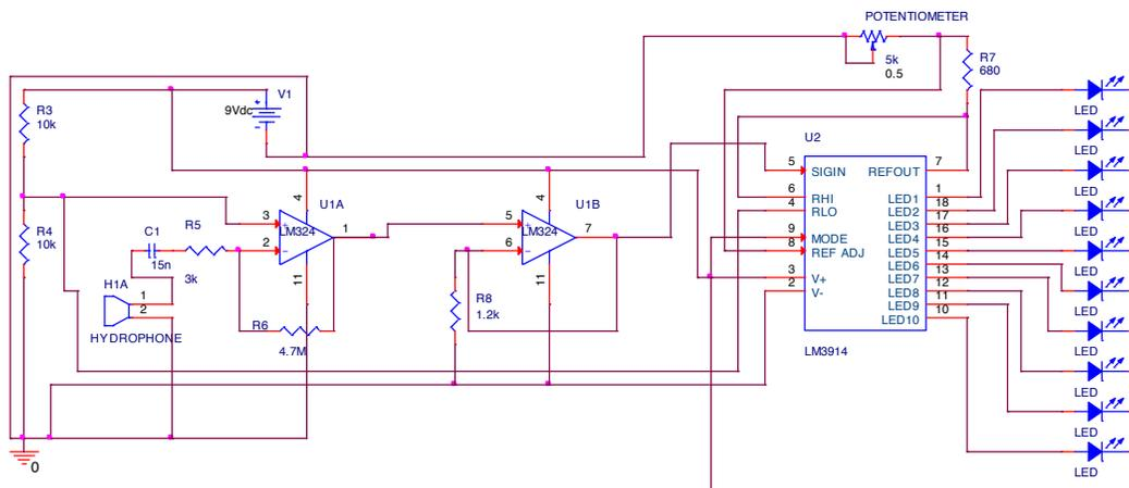
Figure 4 - Electrical system schematic
