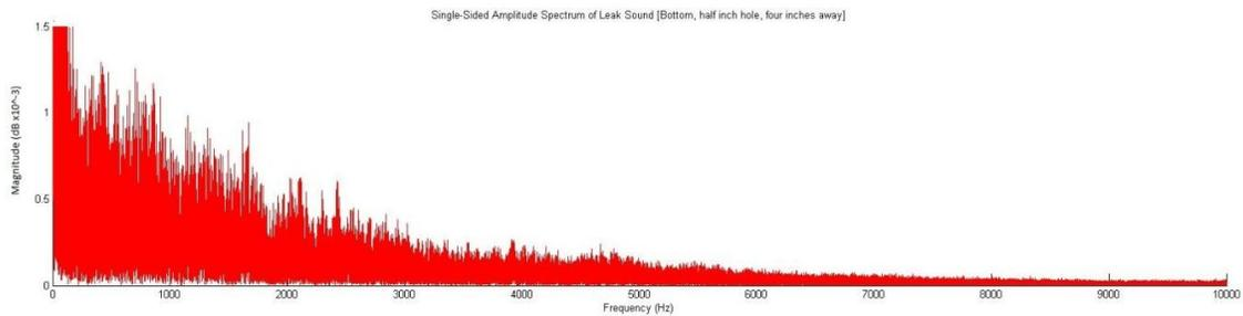
**Figure 5 - Unfiltered amplified leak signal from initial testing**
