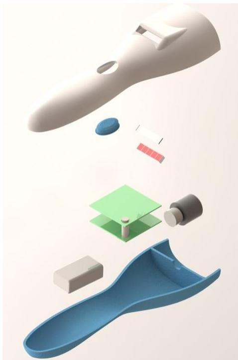
**Figure 7 - Solid model of full-production leak detector concept (exploded view)**
