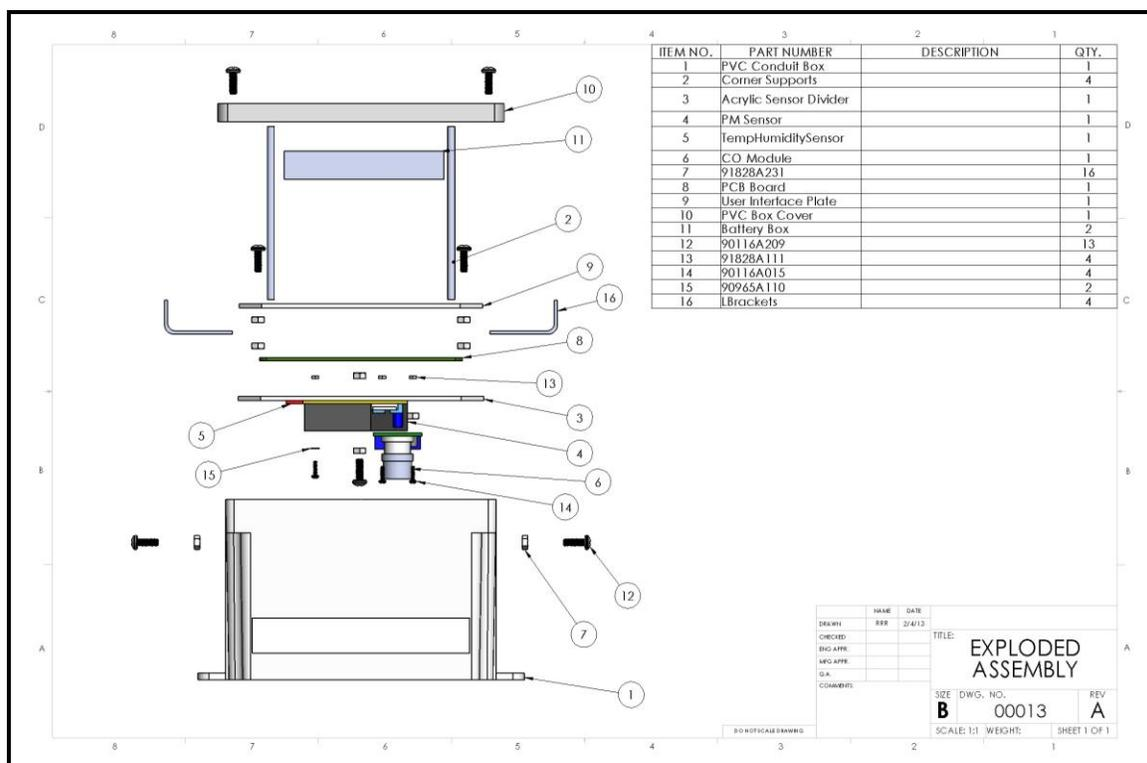
Figure 3: Exploded view of monitor with the bill of materials.
