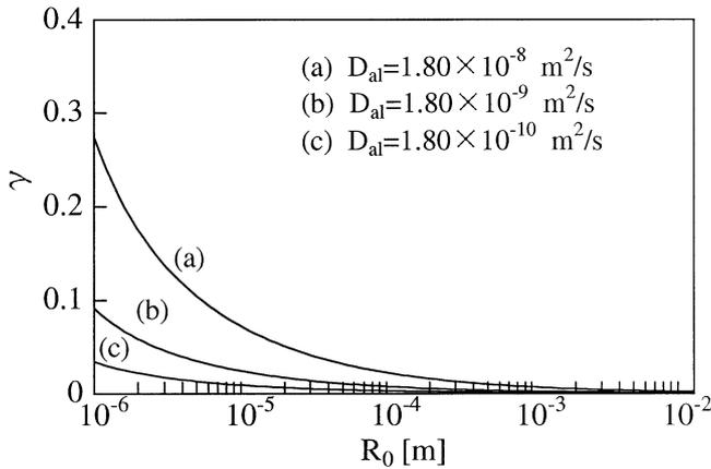
Fig. 5 Diffusion on the decay of bubble oscillation.
