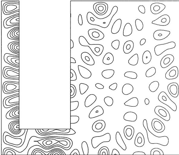
Fig. 11 Isobar diagram in a cleaning vessel,  $le = 6\lambda$ .
