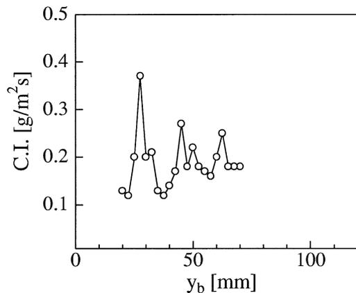
Fig. 15 Cavitation intensity,  $le = 2\lambda$ .
