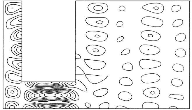
Fig. 8 Isobar diagram in a cleaning vessel,  $le = 4\lambda$ .
