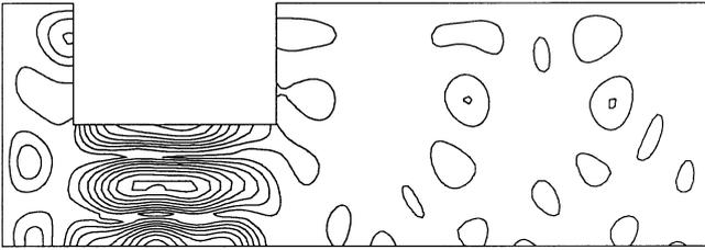
Fig. 10 Isobar diagram in a cleaning vessel,  $le = 2\lambda$ .
