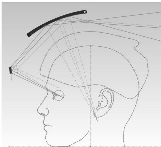
Figure 1. Schematic of geometric optical analysis performed on a proposed dual mirror system.
