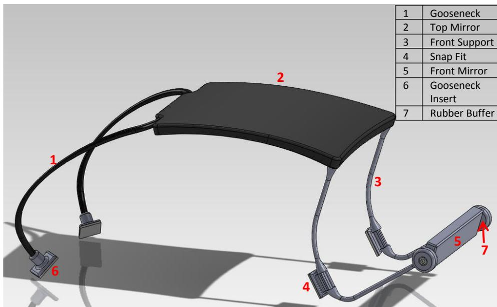
Figure 2. Annotated system assembly.
