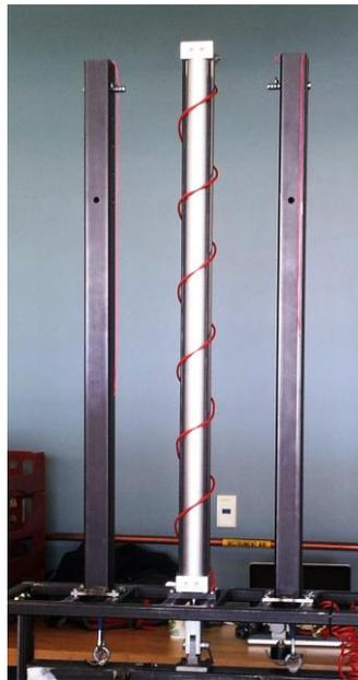
Fig. 1: Springs and Air Piston Assembly
