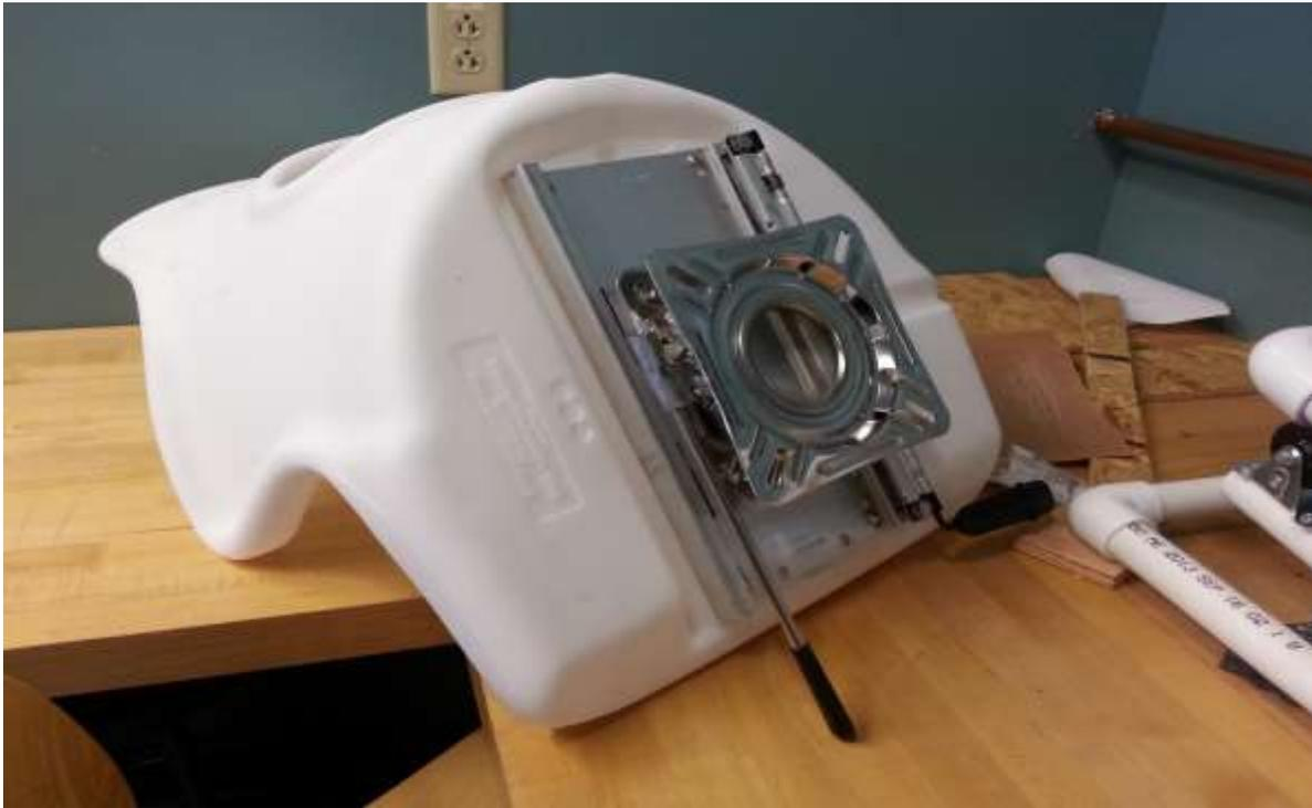
1. Fasten the swivel-sliding mechanism to the bottom of the seat using the four screws included with the mechanism. The rectangular flat plate will have four slots that will be used for fastening these two parts together. The orientation of the seat relative to the swivel-sliding mechanism will be such that the handles will be where the user's legs would be if sitting in the seat.
