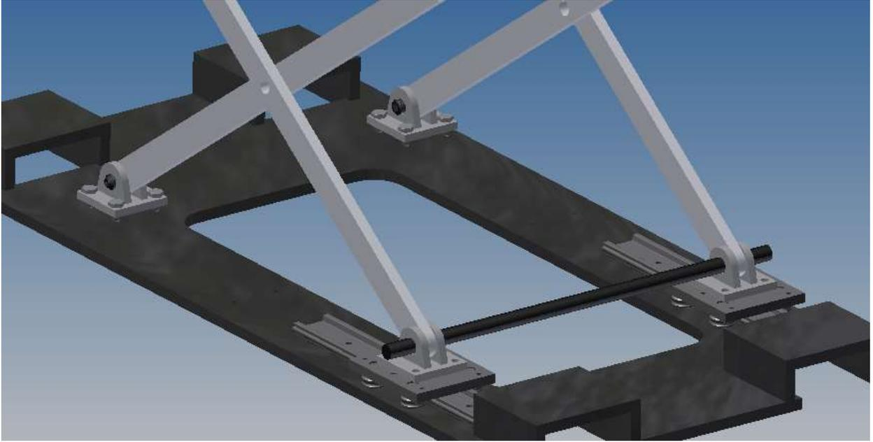
7. The clevises welded to the bottom plate will hold the legs in place. Slide the legs in the clevis slot and secure them with a pin and pin clips.
