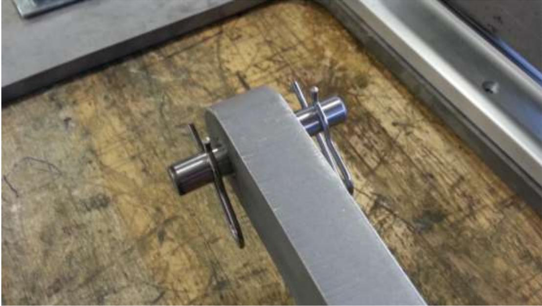
Pin and pin clips will be used in many areas on the device. This is how to use these fasteners. The pin will slide through the holes in the parts being held together and pin clips will fit around grooves in the pins to lock it in place.
