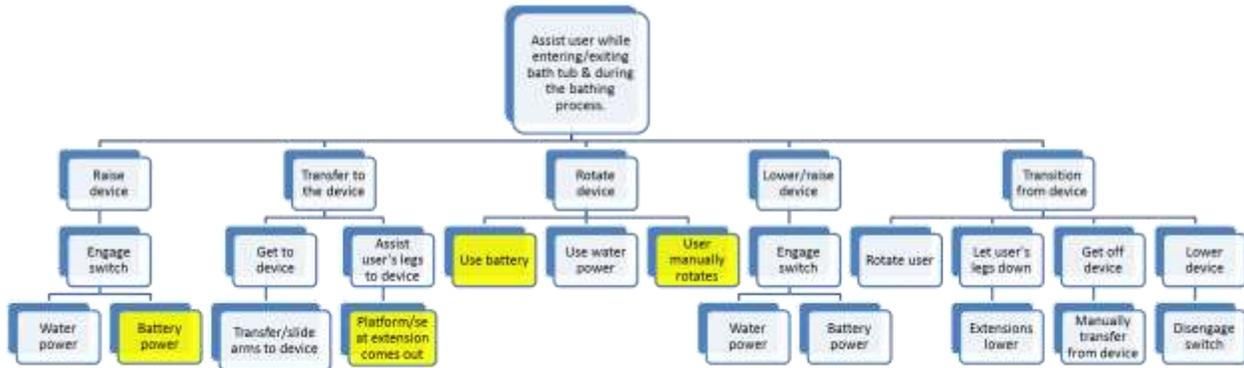
Figure 2: Functional decomposition of the bath tub lift
