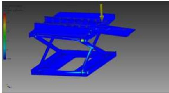
**Figure 6: Stress Analysis at maximum extended position.**
