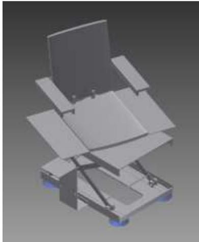
**Figure 4: Conceptual CAD model of the battery powered bathtub lift**
