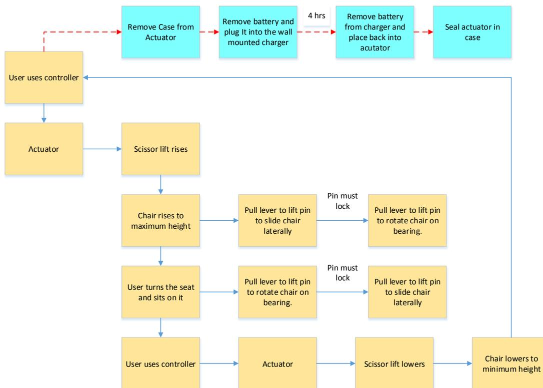
Figure 8: Mechanical architecture of the bath tub lift.
