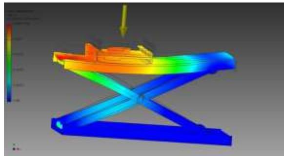
**Figure 5: Displacement analysis showing maximum displacement if 0.03537” while scissor region obtained 0.007-0.023”.**
