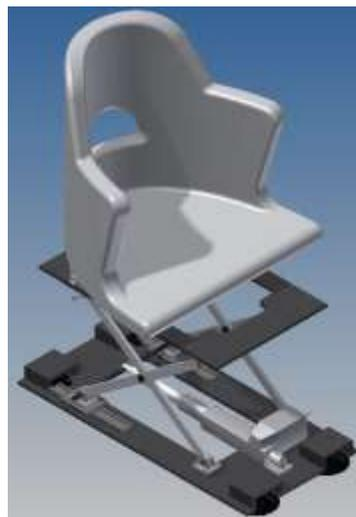
**Figure 7: Final design of the bathtub lift.**
