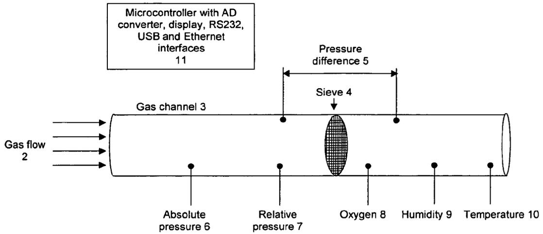
Fig. 2: Gas block in FlowAnalyser measuring device
