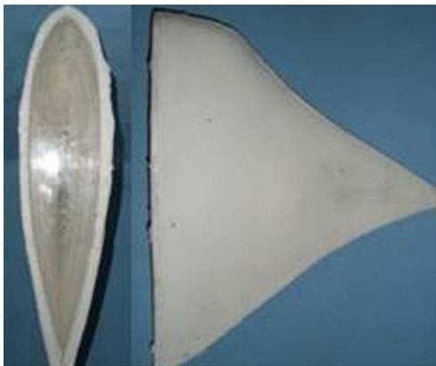
Fig. 4. The right part of the whole-flexible body before dressing, showing with the midsection and the cavity
