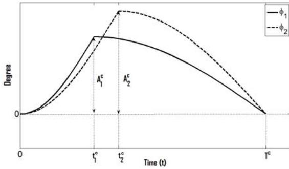
Fig. 14. Prototype of joint angles movements in “C sharp turning” swimming pattern.  $T^c$  is the period of turning,  $A_i^c$  are the amplitudes,  $t_i$  are the switch points between different sinusoid functions.
