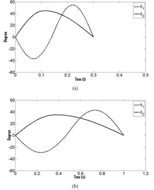
Fig. 15. Joint movement trajectories generated by “cruise in turning” swimming pattern model. (a) Parameters obtained base on observations,  $T^s = 0.3$ ,  $t_1^s = 0.11$ ,  $t_2^s = 0.14$ ,  $A_1^s = 45$ ,  $A_2^s = 37$ , and  $A_2'^s = 55$ . (b) Similar pattern generated by turning parameters,  $T^s = 1$ ,  $t_1^s = 0.37$ ,  $t_2^s = 0.47$ ,  $A_1^s = 35$ ,  $A_2^s = 29$ , and  $A_2'^s = 43$
