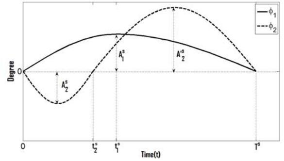
Fig. 11. Prototype of joint angles movements in “cruise in turning” swimming pattern.  $T^s$  is the period of turning,  $A_1^s, A_2^s$ , and  $A_2'^s$  are the amplitudes,  $t_1^s$  and  $t_2^s$  are the switch point between different sinusoid functions.
