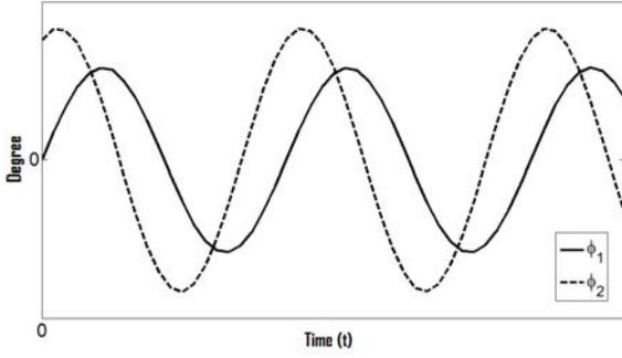
Fig. 8. Prototype of joint angles movements in “cruise” swimming pattern.
