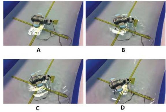
Fig. 18. The robotic fish is swimming in “C sharp turning” swimming pattern.
