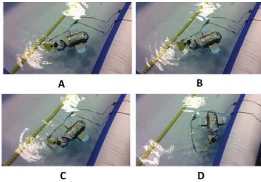
Fig. 17. The robotic fish is swimming in “cruise in turning” swimming pattern.
