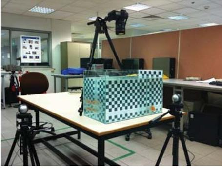
Fig. 4. The video recording system. Three cameras are used simultaneously to record three views, lateral, posterior and overhead. The overhead view is obtained by the high-speed camera, the resolution of every captured image reaches  $1920 \times 1080$  pixels, and the other two views are obtained by two web cameras.
