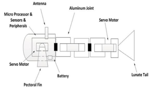
Fig. 2. Structure of the robotic fish.
