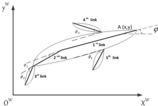
Fig. 1. Multi-joint robotic fish model.
