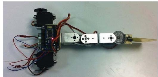
Fig. 3. Framework of the robotic fish without water proof skin covered.
