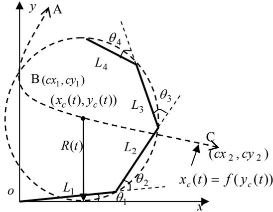
Fig. 5 The joint-end trajectory of C-shape fast turn
