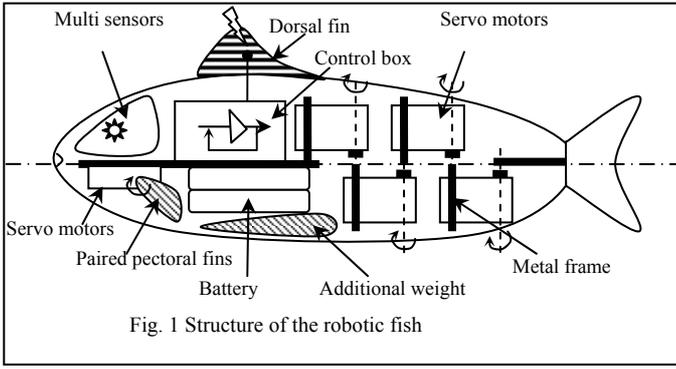
Fig. 1 Structure of the robotic fish
