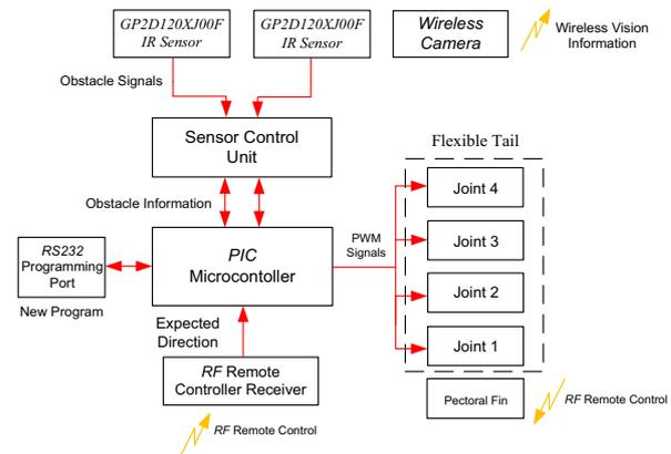
Fig. 8. Drive and control architecture of the robotic fish
