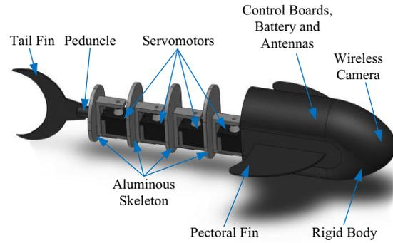
Fig. 7. Mechanical configuration of the robotic fish
