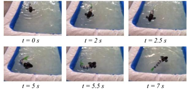
Fig. 11. Swimming of the robotic fish with autonomous-swimming at  $f=2\text{Hz}$
