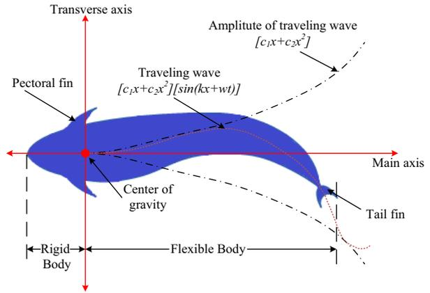
Fig. 1. Physical model of carangiform motion
