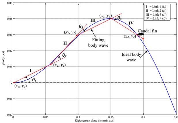
Fig. 3. Body wave curve fitting based on 4-Link flapping mechanism
