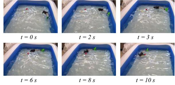
Fig. 10. Swimming of the robotic fish with cruise-turning at  $f=2\text{Hz}$
