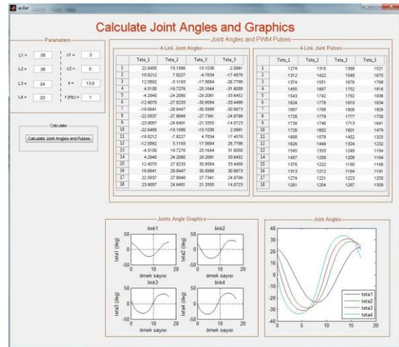
Fig. 4. The interface of the 4-joint flapping mechanism
