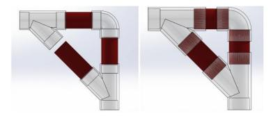
The set time for the PVC primer and cement selected is ~5 minutes, which should allow for enough time for the user to assemble the PVC components and press them together.
