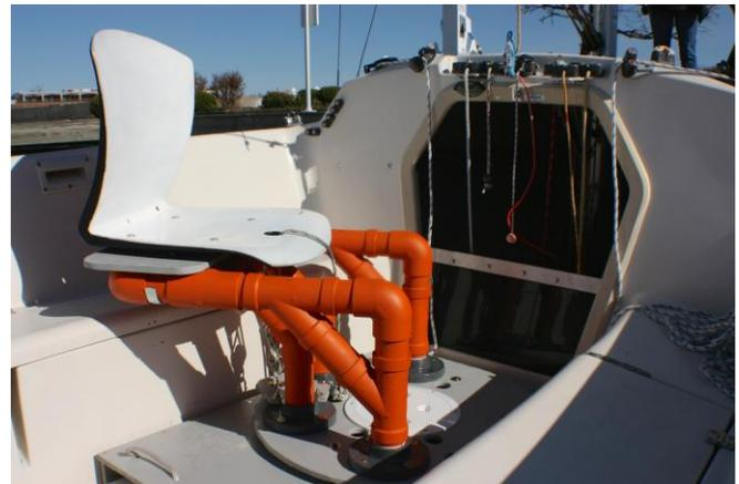
Figure 1 – Jib Transfer System
