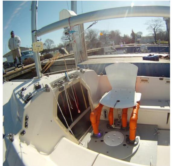
Figure 3 – Jib Transfer System
